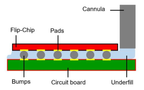
The adhesive has to flow into the narrow gap of less than 100 µm between the silicon and the PCB and encase the individual solder connections. This is achieved using a particularly **low-viscosity adhesive**, the so-called **underfill**.
