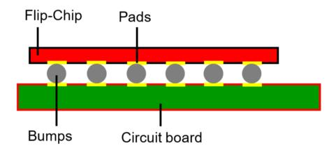
The idea was that these chips could be soldered onto PCBs in the same reflow process as other **SMD** (= **surface mount device**) components. However, this turned out to be **impractical** under today's production conditions for the following reasons:
