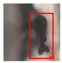
Bond lifted from the bondpad Silver corrosion found under the pad.
