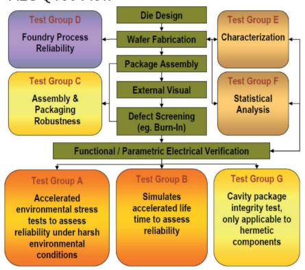
These are all quality assurance procedures to be followed in the design, industrialisation and production of automotive parts that RoodMicrotec can provide.
