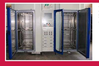
The Burn-in chamber has 2 times 24 slots (Burn-in board positions), each of the chambers (left and right side) can run at an independent temperature, and every slot can run with a different product. This results in maximum 2 times 24 different products at two different temperatures to be processed in parallel.
