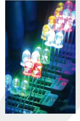
Selection tests are essential, because the human eye is for example very sensitive to brightness and colour in car displays or washing machine displays.
